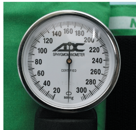
Figure 20-10 A. A manual sphygmomanometer consists of a cuff, a bulb, and a manometer. The manometer may be either aneroid or mercury. Do you know which type of manometer is shown here? The tubes attach the inflatable pouch inside the cuff to the bulb and to the manometer. B. An aneroid manometer. C. A mercury manometer.
